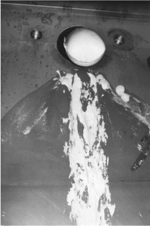
Figure 4 Butter is discharged into the covered silo.
