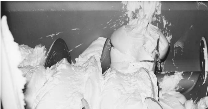
Figure 5 Butter in covered silo moving to a rotary positive displacement pump by augers.
