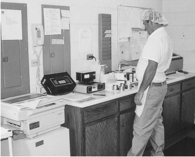
Figure 5 QA/receiving technician screens incoming raw milk for antibiotics/inhibitory substances. (Photograph courtesy of Mayfield Dairies and Dean Foods Company, Athens, TN.)
